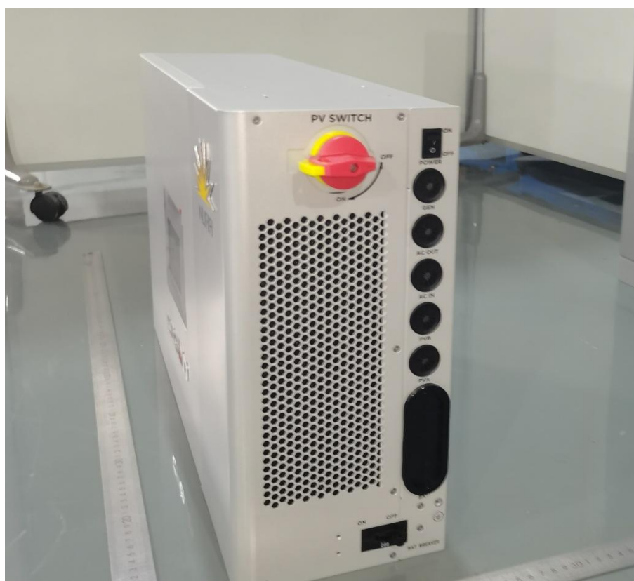
Fig. 7 -- Side view (inverter)
