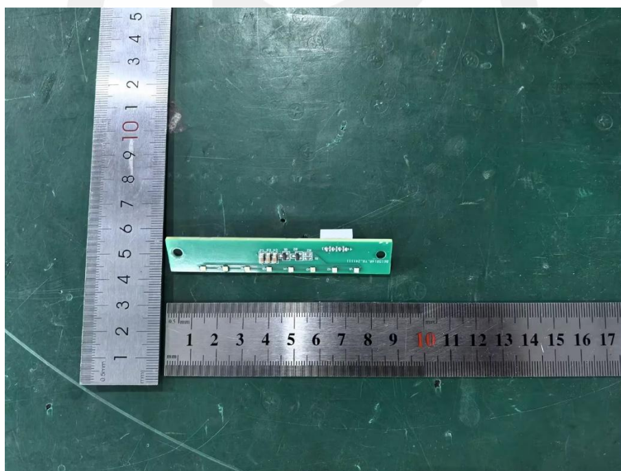
Fig. 18 --LED board view 2
