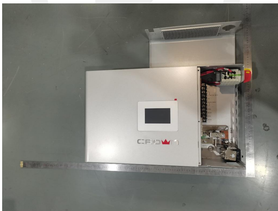
Fig. 8 -- Interior view (inverter)
