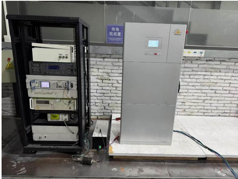
16.9. Photo of Magnetic Field Immunity Test
